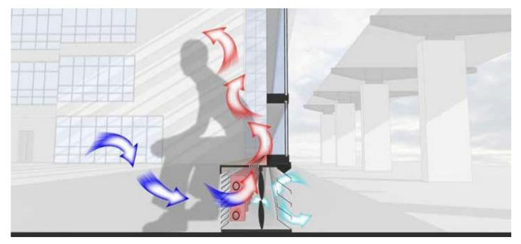
In winter, louvers inside the bench close with the heaters on – this design warms a minimum amount of cold fresh outside air, while heating and recalculating the cold air at the perimeter windows of the space.
