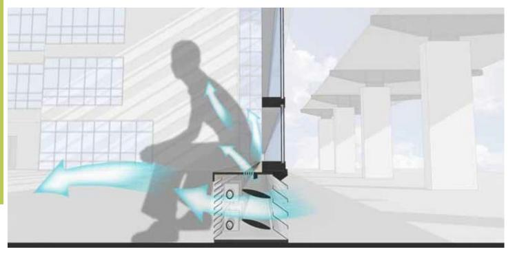
In summer, louvers inside a bench open with the heaters off, allowing a maximum amount of fresh outside air to naturally ventilate the interior space
