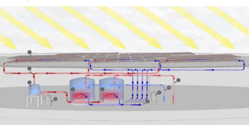
method, while common in the design-build solar market, offers the least desirable alternative, as it shortens the life of components and can result in hot glycol discharging from relief valves if pressures exceed allowable limits. Glumac doesn't recommend this approach.
